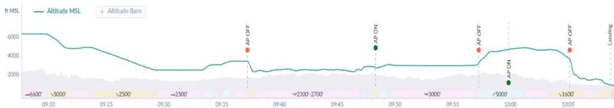
Fig. 1 – Flight altitude profile of VL 3 UL aircraft, registration mark I-B866, in FIR PRAGUE during flight from Italy
