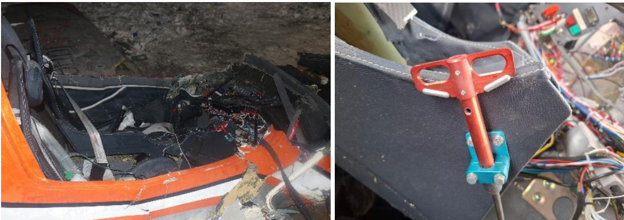
Fig. 13 – Unlocked rescue system activation control
